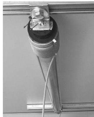
Even without tension the cable wraps are neatly side by side and no overlapping.
