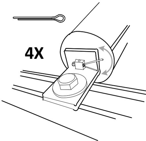
Tighten screw until the washer no longer rotates. Then tighten screw another 135° in the same direction.
