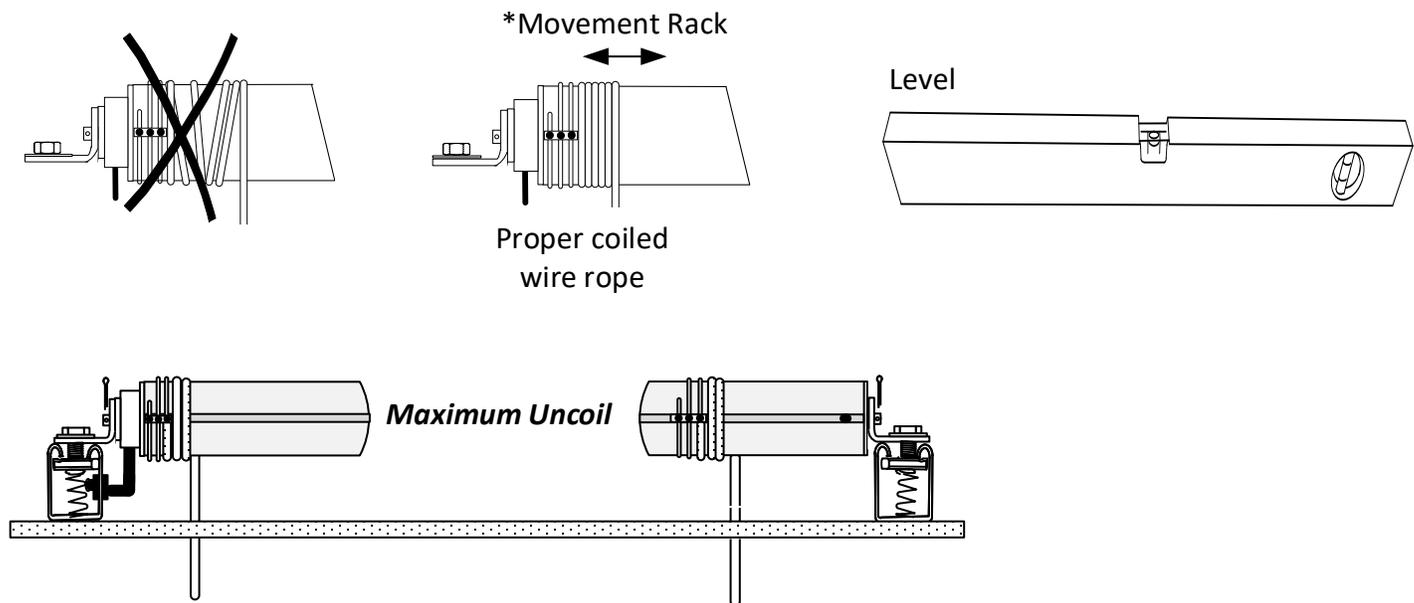
**Adjustment is only possible with the DeadMan switch OFF, and after a motor limit has been reached or lift is stopped manually (white LED lights on controller are lit and stay on).**
