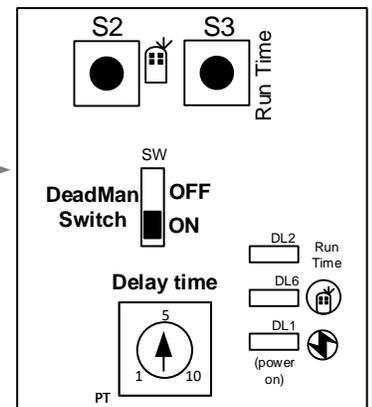
**DeadMan Function:** You use only the UP and DOWN buttons. You have to hold the button to make the lift move. When you release the button the equipment will stop immediately. If a key gets jammed you can stop the equipment with the stop button.
