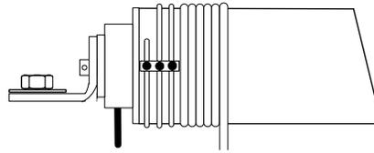
Proper coiled wire rope
