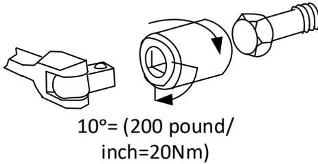
**Tighten screw until the washer no
