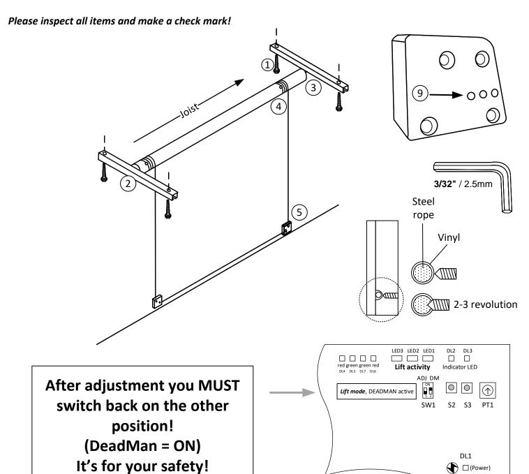
Important! The Lift has to run to the ceiling end points (stopped automatically) in order to be leveled properly.
