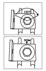
Tighten screw until the washer no longer rotates. Then tighten screw another 135° in the same direction.
