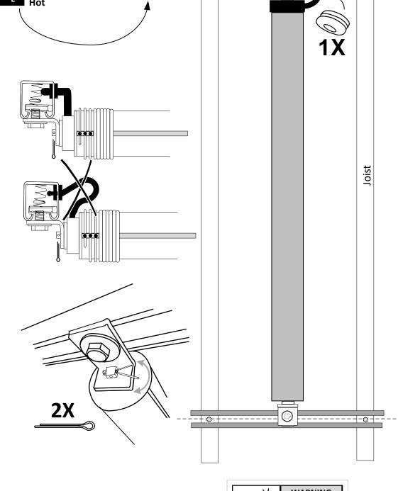
Note the use of grommets and the wire path into the strut
