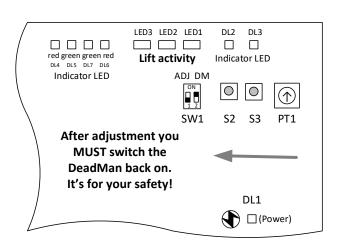
**DeadMan Function:** You use only the UP and DOWN buttons. You have to hold the button to make the lift move. When you release the button the equipment will stop immediately. If a key gets jammed you can stop the equipment with the stop button.
