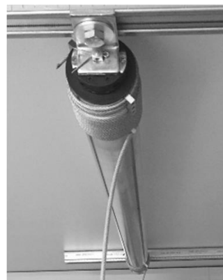
Even without tension the cable wraps are neatly side by side and no overlapping.
